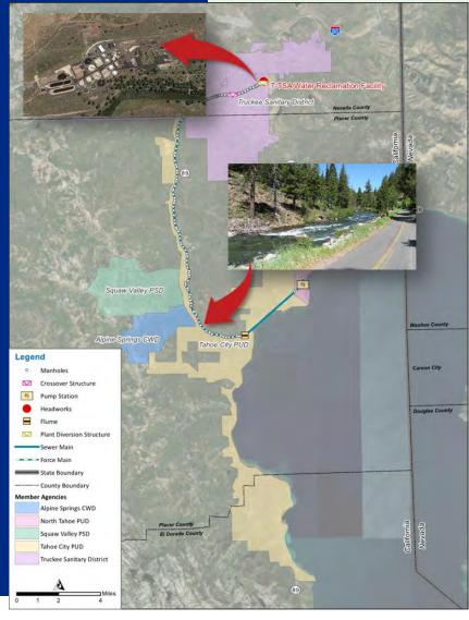
The TRI extends from its southern reach in Tahoe City to the WRP, and runs exclusively along the Truckee River. It ranges in size from an 24" to a 48" gravity sewer and is constructed almost exclusively of reinforced concrete pipe. The corridor is narrow and limited in terms of options for additional conveyance capacity, and construction or rehabilitation is complicated and expensive.
