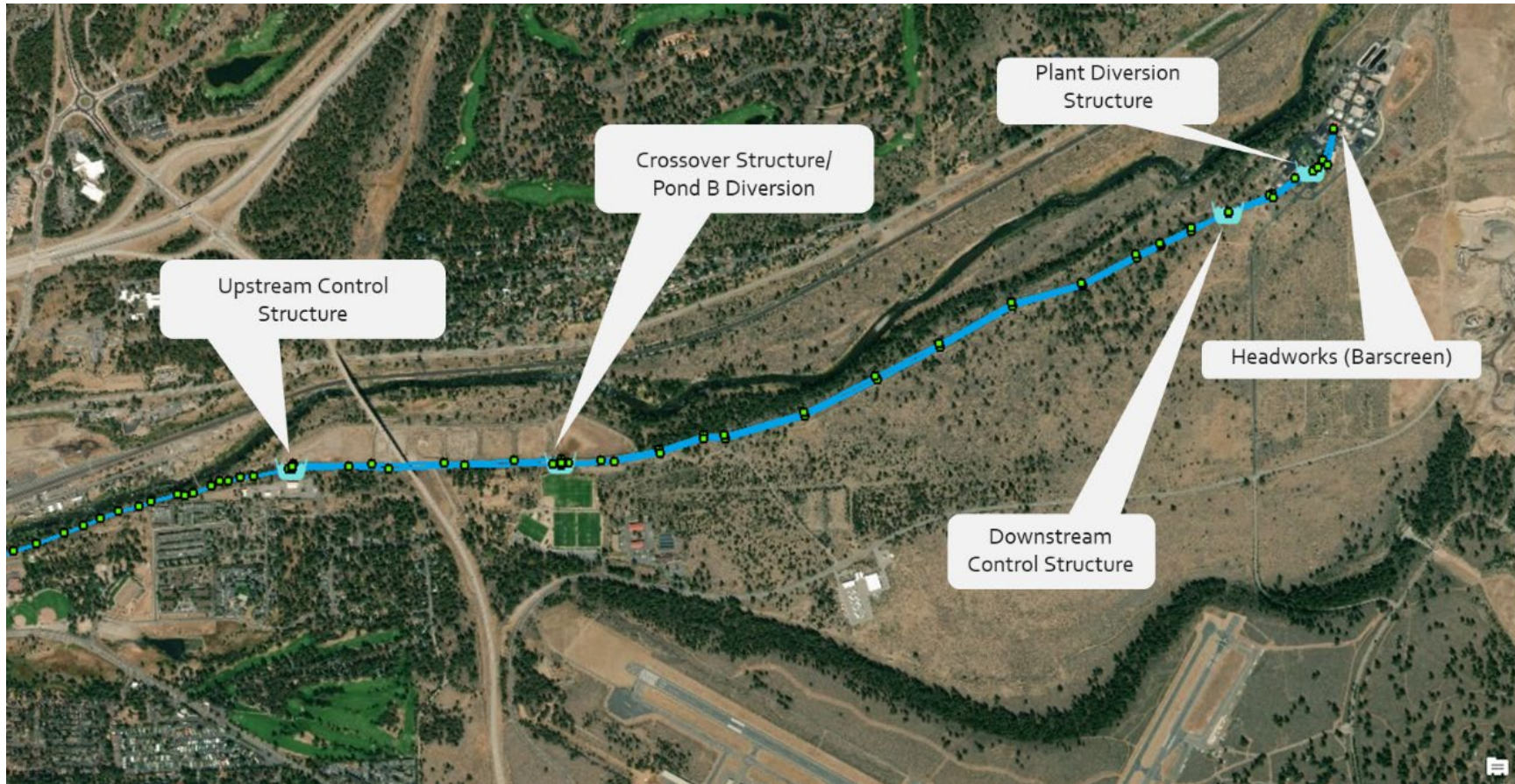
Figure 4.2 Special Structures in TRI Hydraulic Model
