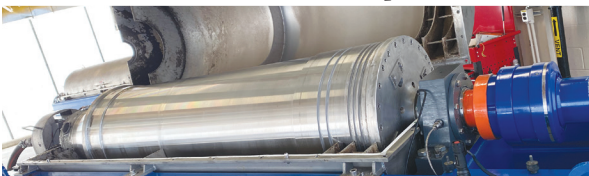
"Sludge Dewatering Centrifuge"
