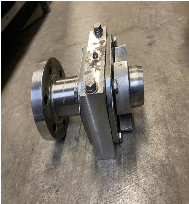
Cake Conveyor Intermediate Bearing
