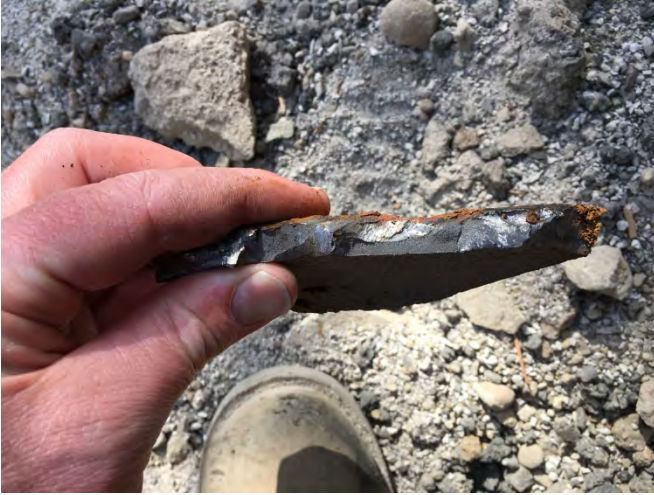
Photo 1 – 40 Year Old Ductile Iron Fragment
